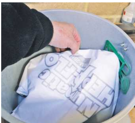
▲ The first filter is the collection bag; you can use the vac without one though
